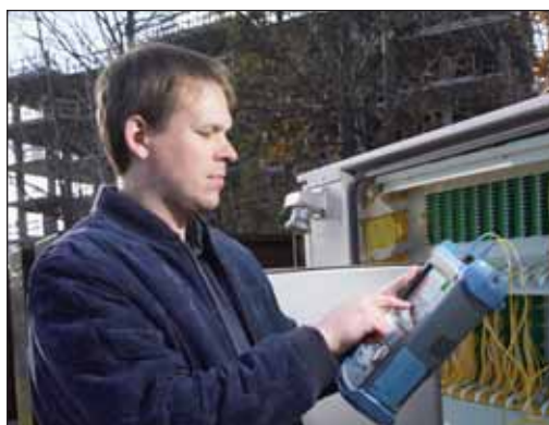
Perform full averaging in 45 seconds with the short-range OTDR configurations.
