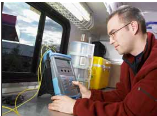
Long-range OTDRs display high-speed traces in as little as 10 seconds.
