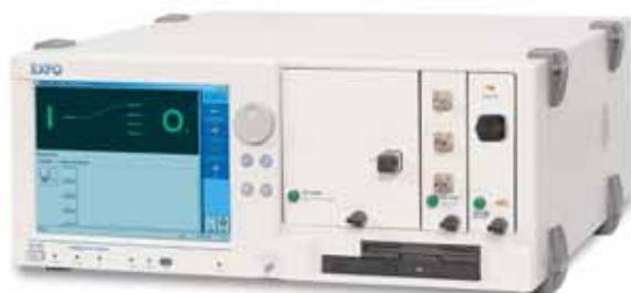
An IQS-9100 Optical Switch, an IQS-5250B Optical Spectrum Analyzer and an IQS-1600 High-Speed Power Meter combined with an IQS-505P five-slot controller
