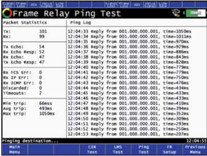
A Frame Relay Ping Test
